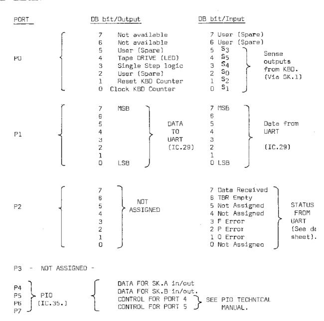
REMAINDER (P8—PFF): Higher level port decoding will be on the expansion board so with the "PORT SELECT" link (LK.1) on the CPU PC8 set to "INTERNAL" the above group of 8 addresses will be found to repeat a total of 32 times up to the total 256 Port addressing capability of the Z80 CPU.
