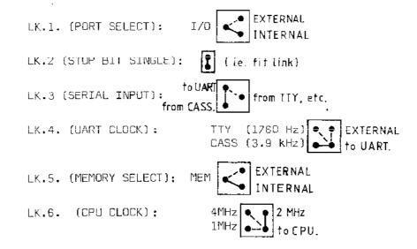
Fit only one wire per link as shown by the thick lines. The dotted lines indicate alternative connections.
